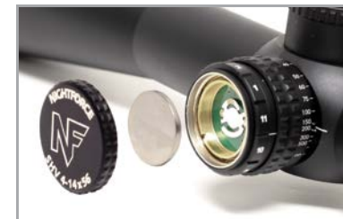
Unscrew the outer cap counterclockwise to change the battery.
