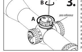
A) Turn the dial counterclockwise until the "0" on the dial is aligned with the fixed zero reference mark below. B) While holding the dial, tighten both set screws to 4 inchpounds. If you don't have a torque driver, use the Allen wrench, holding the short end of the wrench while turning to prevent overtightening.
