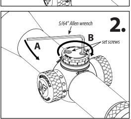
A) While holding the adjustment dial, loosen the two set screws on top of the dial using the supplied 5/64" Allen wrench. The dial should now rotate freely, and you should not feel any clicks. B) Rotate the dial clockwise until it stops.
