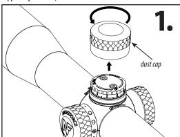
Zero your riflescope with your chosen load (see instruction manual). To then reset the number scale to 0, remove the dust cap by rotating it counter-clockwise.
