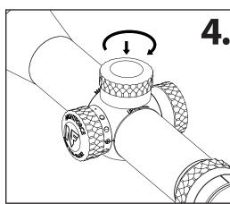
A) Turn the dial counterclockwise until the "0" on the dial is aligned with the fixed zero reference mark below. B) While holding the dial, tighten both set screws to 4 inchpounds. If you don't have a torque driver, use the Allen wrench, holding the short end of the wrench while turning to prevent overtightening.
