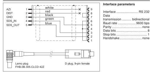
The optional interface cable is intended for connection to a PC serial interface with a 9-pin D plug.
