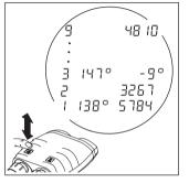
Click azimuth key repeatedly to obtain the last nine measurements in succession.
