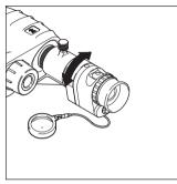
Carefully slide the night vision device into the adapter and clamp it using the knurled locking screw. At observation distances below 100 m, focus the night vision device by rotating its casing.
