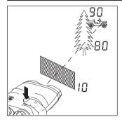
Up to 3 separate distances can be obtained with a single measurement, for example when:
