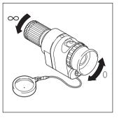
Activate the "niGt" function in the configuration menu (see pages 24, 25). Remove the eyecup from the right eyepiece. Rotate the right eyepiece to adjust it to 0 dioptres. Then slide the eyepiece fully inwards. Fit the adapter, and screw it firmly to the tripod bush.
