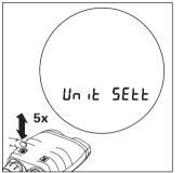
Various angle and distance measurement units may be set via the configuration menu.
