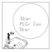
Click the azimuth key six times in rapid sucession to store the setting.
