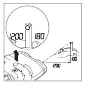
Release the distance key while holding the VECTOR steady. The horizontal distance appears at the left and the height difference at the right of the field of view.
