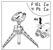
Place the VECTOR on mini-tripod SST3-2 or equivalent and level 30° downwards (see marking on tripod).
