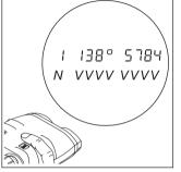
Automatically, the last measurement appears, identified by the number "1" at the very left. Explanation of display: N=Number of measurement (1-9) "1" = last measurement "2" = second but last, and so on
