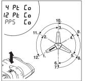
Now press the distance key until "PPS Co" is displayed. The calibration procedure starts automatically in a few moments. Proceed as described before. As a help for "rot 60°": rotate from the first tripod foot to the middle position between this and the next foot, then to the next foot and so on.
