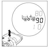
The distance display blinks for a few seconds after a multiple distance measurement. Click the distance key repeatedly to obtain all the measured distances in succession.
