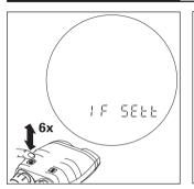
Various interface settings can be set. Click the azimuth key six times in rapid succession. "IF SEtt" appears briefly in the field of view, followed by the current setting.
