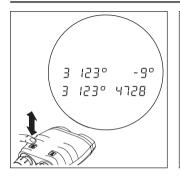
While showing a combined "Distance/Azimuth/Inclination" measurement, azimuth (left) and slope distance (right) appear first. Click azimuth key again to obtain inclination (right) and azimuth again (left). As it is the same measurement, the number N at the very left does not change.
