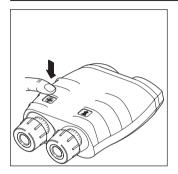
Press and hold the azimuth key. The current azimuth appears. The display updates twice per second.
