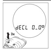
Click the azimuth key three times in rapid succession. The stored declination value is displayed.
