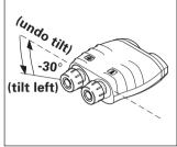
The VECTOR needs to be swivelled in various directions during calibration. Instructions for the required direction of movement appear successively in the display:
