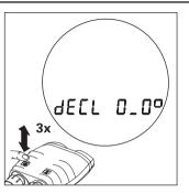
Click the azimuth key three times in rapid succession. The current declination value is displayed for 10 seconds. The VECTOR displays "Old dECL" before switching itself off (the declination value is unchanged). Declination is displayed in the currently selected angular units (see page 28).
