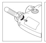
Open the battery compartment using a suitable tool, or a coin. Insert a 6V lithium battery, type 2CR5 or equivalent. Ensure that the drawing ribbon lies above the securing tape of the battery cover. Keep the battery cover seals and the instrument case clean.
