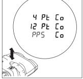
If you want to perform the 12 point calibration click the distance key when "4 Pt Co" is displayed until the desired option is displayed. The selected procedure starts automatically in a few moments. Move the VECTOR according to the displayed instructions (see page 34).
