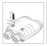
Click the azimuth key once, then immediately press and hold it down.
