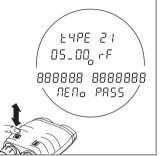
Use the azimuth key to scroll through the list.
